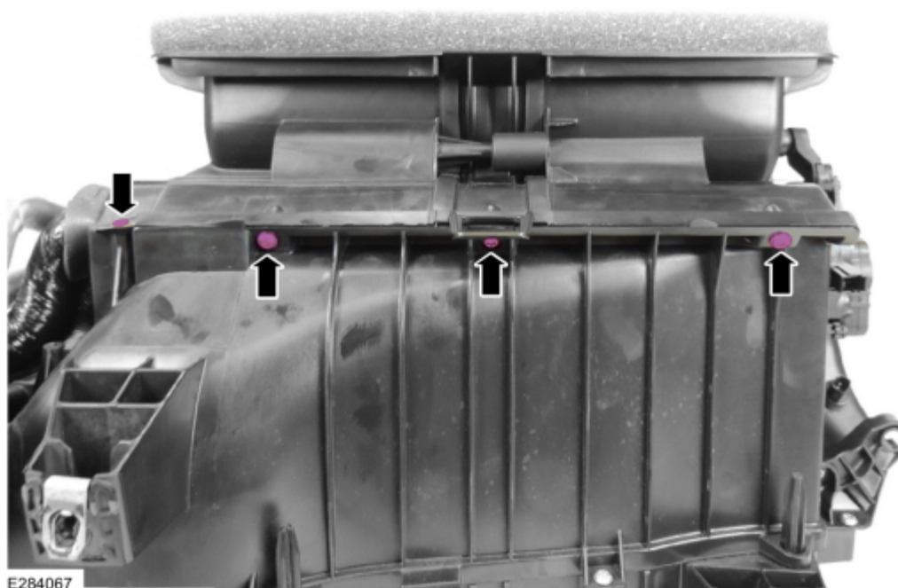
13. Position the bulkhead insulator over the thermostatic expansion valve (TXV). (Figure 12) Figure 12
